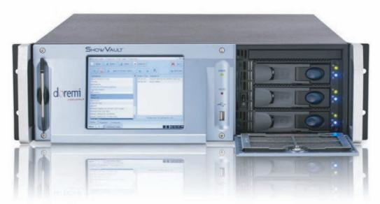
Doremi's new ShowVault is a dedicated storage server capable of playing JPEG2000 digital movies that conform to DCI specifications. ShowVault was specifically developed to interface with Doremi's IMB (Integrated Media Block) which is available inside Series 2 DLP projectors making 2K & 4K playback possible.
